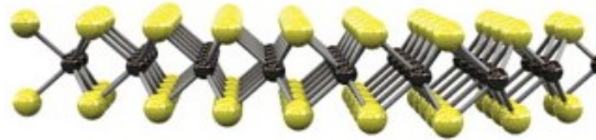
Figure 1: Structure of a monolayer Transition Metal Dichalcogenide as seen from the side, with the black dots representing the transition metal atoms (M) and the yellow dots representing the chalcogen atoms (X) [5].
