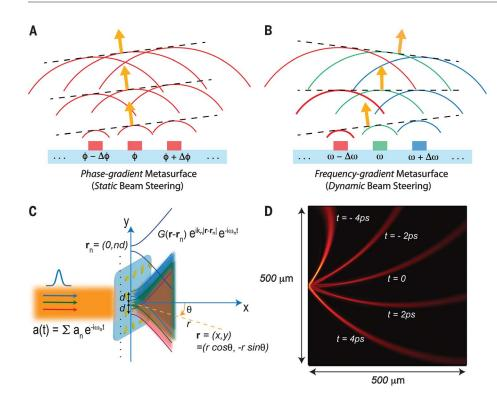
Fig. 1. Theoretical concept behind the proposed frequency-gradient metasurfaces.
