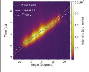
Fig. 3. Experimental results of the beam-steering action.
